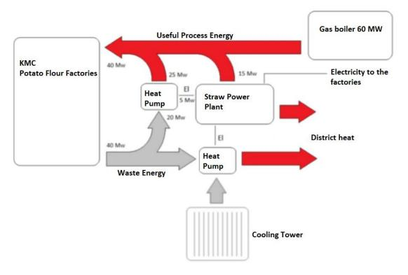
Heat pumps are integrated in the straw power plant and absorb waste heat after the factories or by cooling air in cooling towers. District heating towns in the catchment area of Brande are supplied with district heating see
